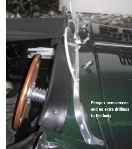
Perspex aeroscreens and no extra drillings to the body
